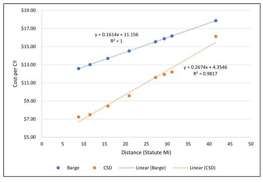
Figure 16. Dredged Fill Unit Cost (\$/CY) (Ph. 2 Sand Transport from Tiger Pass Stockpile)
