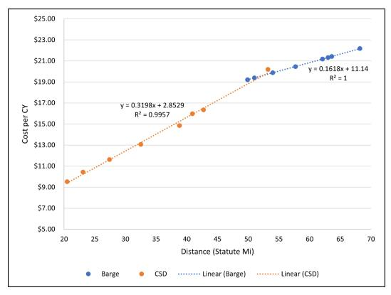
Figure 18. Dredged Fill Cost Unit Cost (\$/CY) (Direct to Island Sand Transport)
