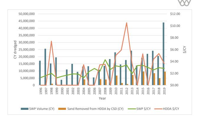
Figure 6: Comparison of total Southwest Pass dredged volumes and dredging unit costs to HDDA volumes and dredging unit costs for 1996-2019.
