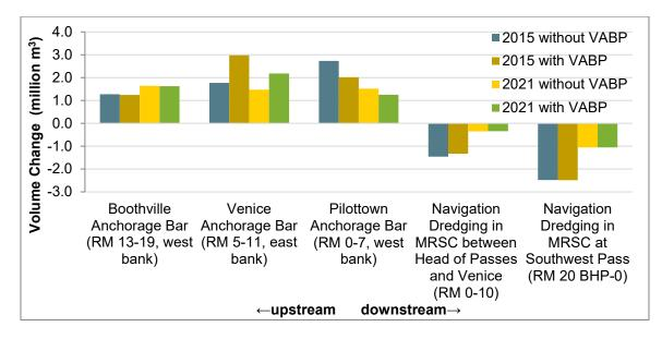
Figure 8. Volume changes at sand bars and dredged volumes from the MRSC between Venice (RM 13) and SWP (RM 20 BHP) for scenarios without and with the Venice Anchorage Borrow Pit (VABP, RM 8) for 2015 and 2021 hydrographs. From Georgiou et al. (2023).
