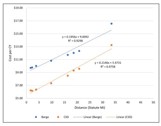
Figure 17. Dredged Fill Unit Cost (\$/CY) (Ph. 2 Sand Transport from Scofield Stockpile)
