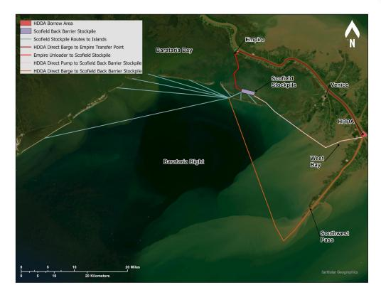
Figure 12. Scofield Island sand stockpile alternatives group.
