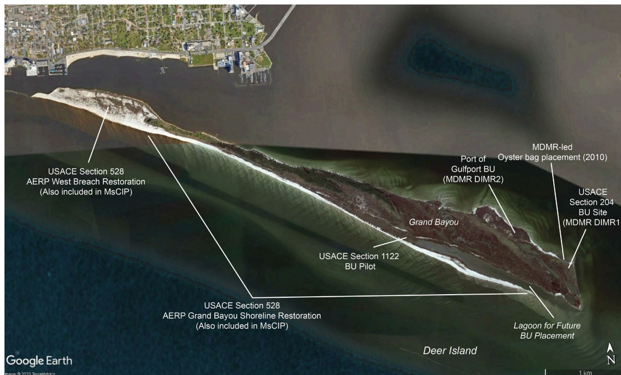
Figure B-2. Natural and Nature-Based Features at Deer Island, Mississippi. Shown are projects authorized under WRDA 2000 Section 528 as Aquatic Ecosystem Restoration Projects (AERP) and later incorporated into the Mississippi Coastal Improvements Program (MsCIP) comprehensive plan; beneficial use (BU) projects authorized under WRDA 1992 Section 204 and WRDA 2016 Section 1122; BUDM sites DIMR1 and DIMR2 filled with dredge material from the Port of Gulfport navigation deepening project; and project led by the Mississippi Department of Marine Resources (MDMR) to place bags of oysters as part of a living shoreline approach.
