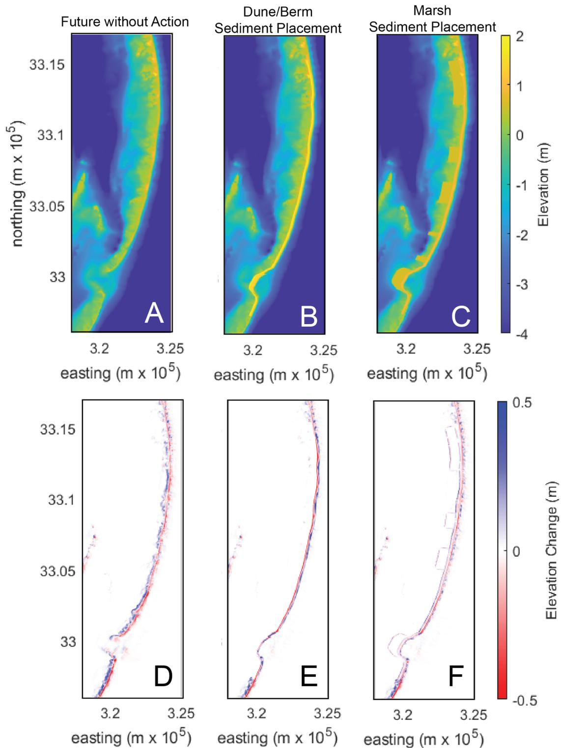
**Figure 44. Pre-storm elevation for the FWOA (A), dune/berm sediment placement (B), and marsh sediment placement (C), along with the change in elevation during a strong storm event with waves from the SE (D-F for FWOA, dune/berm sediment placement, and marsh sediment placement, respectively).**
