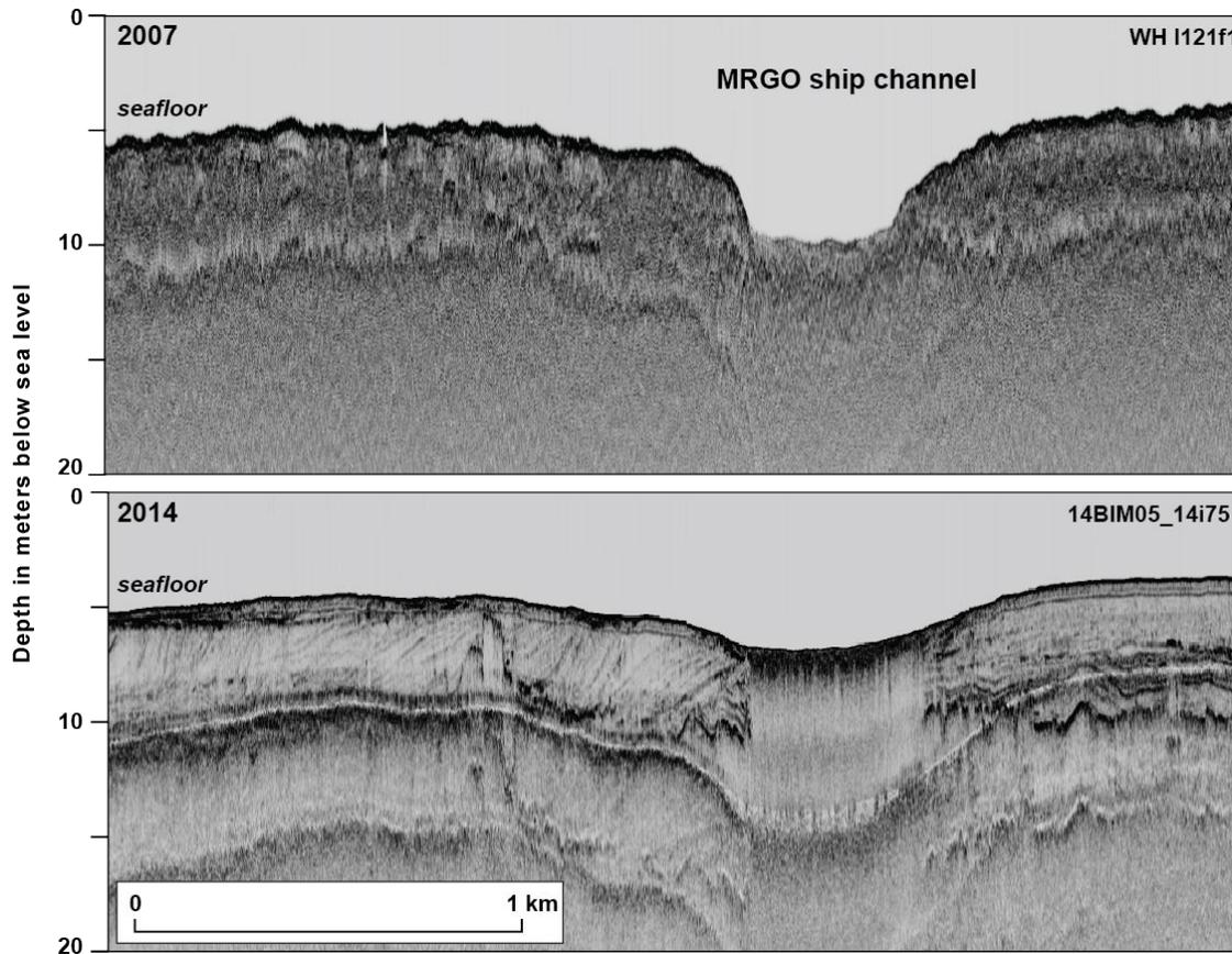
**Figure 12.** Chirp sonar subbottom profiles from 2007 with the exact same transect reoccupied in 2014 crossing the Mississippi River Gulf Outlet (MRGO) navigation channel. MRGO was decommissioned in 2008. Note the infilling in the 2014 profile versus the 2007. From Flocks et al. (2015).
