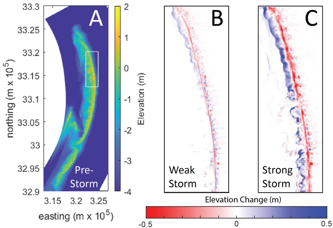
**Figure 39. (A) Pre-storm DEM and the pre- and post-storm elevation change for the region shown in white. Results are shown for a weak (B) and strong (C) storm with shore normal waves.**
