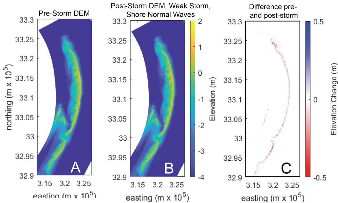
**Figure 35. Pre-storm (A) and post-storm (B) DEM for a weak storm with shore-normal waves (Table 3), along with the elevation change (C) during the storm.**
