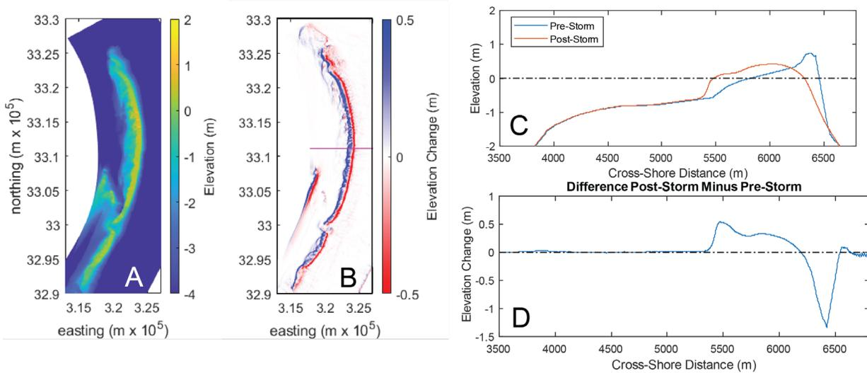
**Figure 47. Post-storm elevation (A) and elevation change (B) for an extreme storm impacting the FWOA case. Also shown are a pre- and post-storm profile (C) and the elevation change during the storm (D) for the profile shown in pink in (B).**
