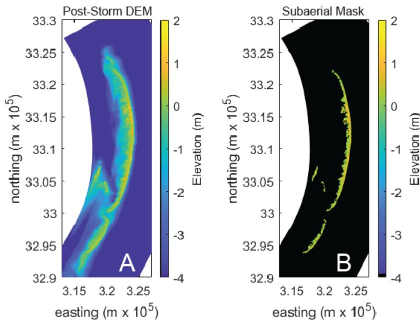
**Figure 29. (A) Post-storm DEM for a low-intensity storm with incident on-shore waves. (B) To calculate the post-storm subaerial volume, areas with elevation less than -0.17 m mean low water**
