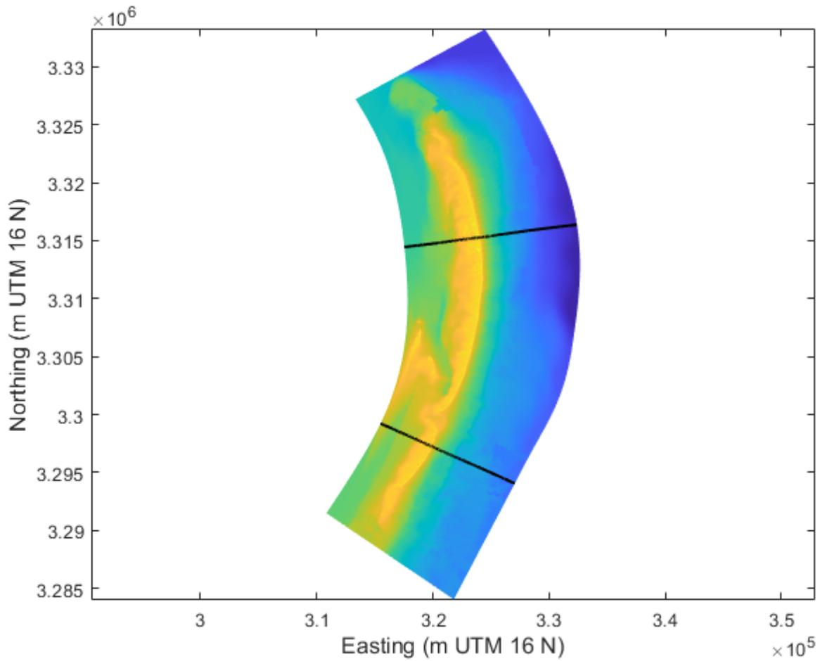
**Figure 22. The model grid of the Chandeleur Islands with the restoration area shown. Between the two black lines the restoration profiles were applied.**
