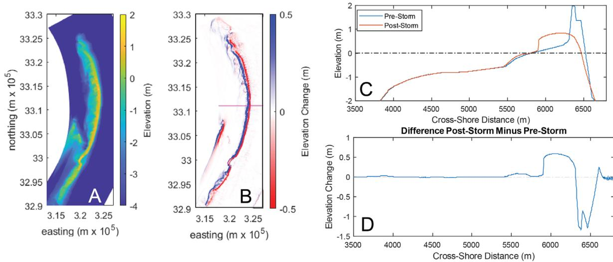
**Figure 49. Post-storm elevation (A) and elevation change (B) for an extreme storm impacting the dune restoration case. Also shown are a pre- and post-storm profile (C) and the elevation change during the storm (D) for the profile shown in pink in (B).**
