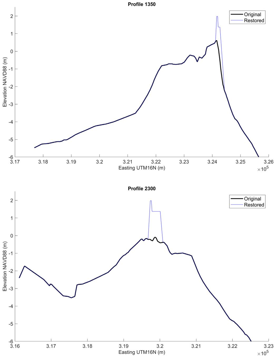
**Figure 24. The dune template applied to topo-bathy profiles. Top: The dune template applied through the restoration area, except for Katrina Cut. Bottom: The dune template applied at Katrina Cut.**
