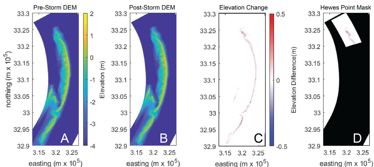
**Figure 31. Calculation methodology for VHewes, the net volume of sediment transported to Hewes Point. The difference between the pre-storm (A) and post-storm (B) elevation is taken (C), then the net sediment volume change is calculated in the region of Hewes Point (D) with the rest of the domain masked out (in black).**
