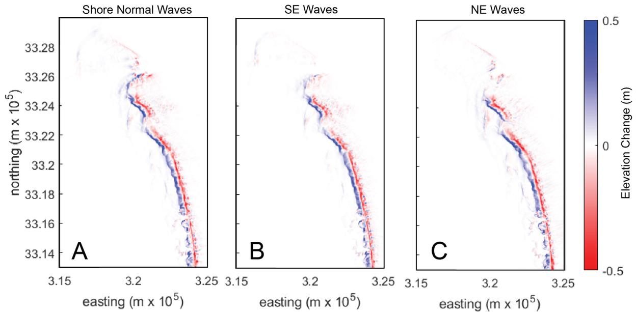
**Figure 37. Elevation change along the northern half of the island chain and at Hewes Point resulting from a strong storm with shore-normal waves (A), waves coming from the SE (B), and waves coming from the NE (C).**
