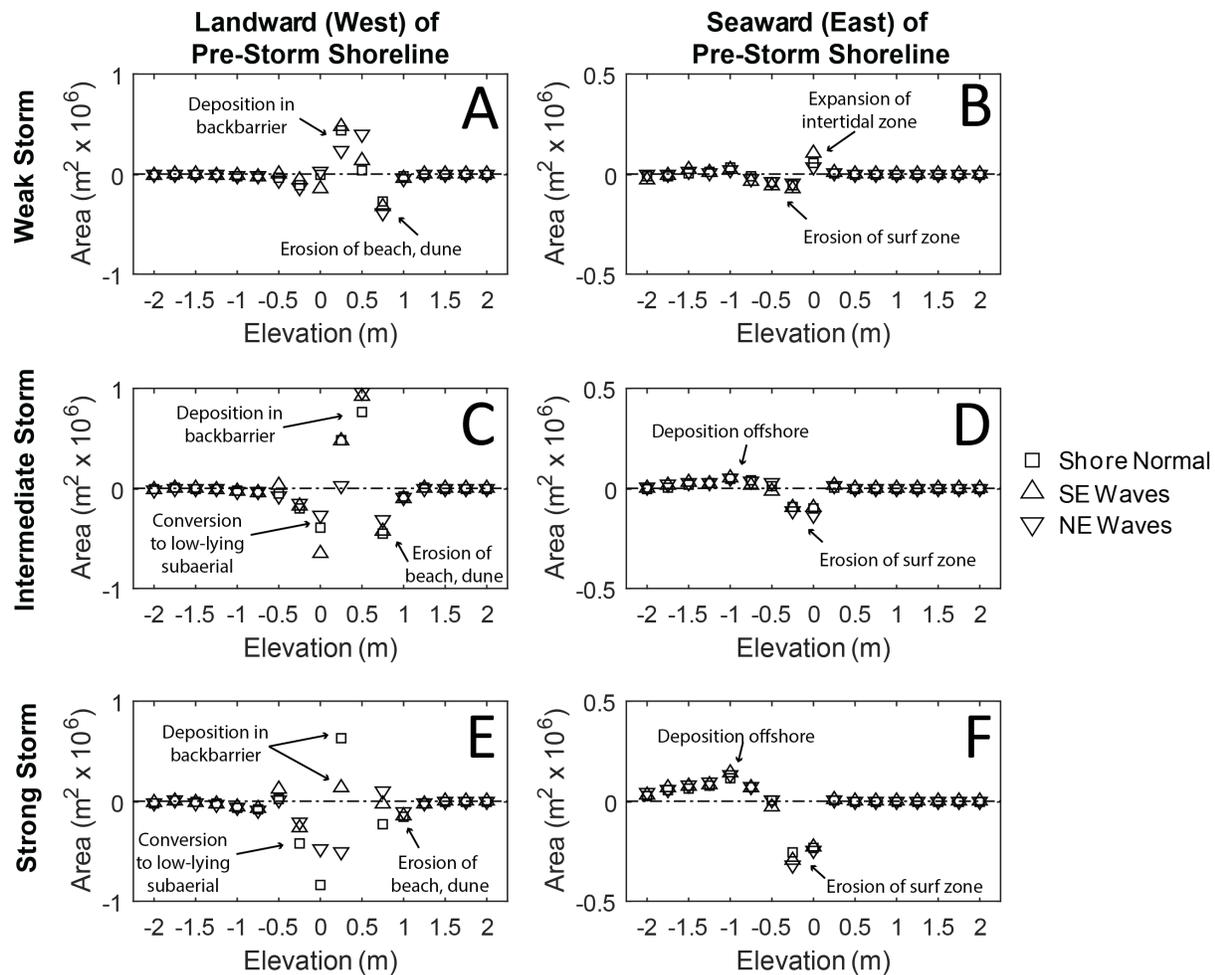
**Figure 43.** Change in distribution of shallow and subaqueous elevation by area pre- and post-storm for a weak (A, B), intermediate (C, D), and strong (E, F) storm. The column to the left shows the change in area landward of (west) of the pre-storm shoreline and the column to the right shows area change seaward (east) of the pre-storm shoreline.
