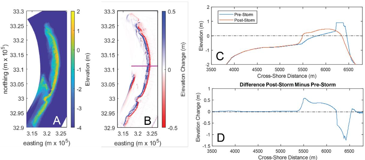
**Figure 48. Post-storm elevation (A) and elevation change (B) for an extreme storm impacting the marsh restoration case. Also shown are a pre- and post-storm profile (C) and the elevation change during the storm (D) for the profile shown in pink in (B).**
