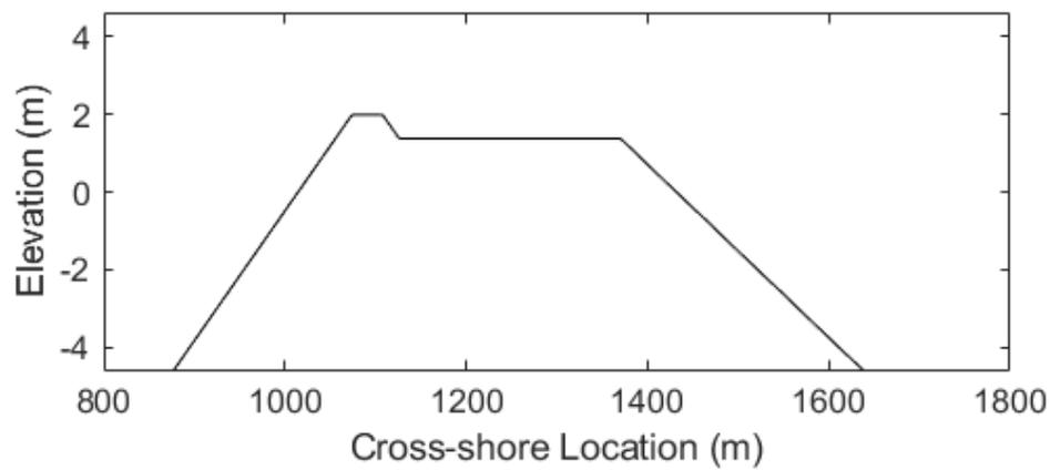
**Figure 23. The dune end member restoration template. Top: The dune and beach template applied to most of the profiles. Bottom: The dune and beach template applied in Katrina Cut.**
