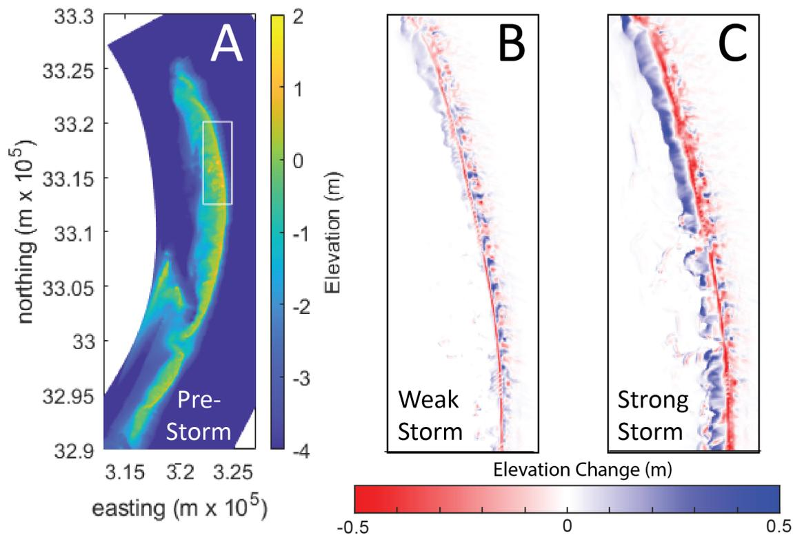
**Figure 40. (A) Pre-storm DEM and the pre- and post-storm elevation change for the region shown in white. Results are shown for a weak (B) and strong (C) storm with SE waves.**
