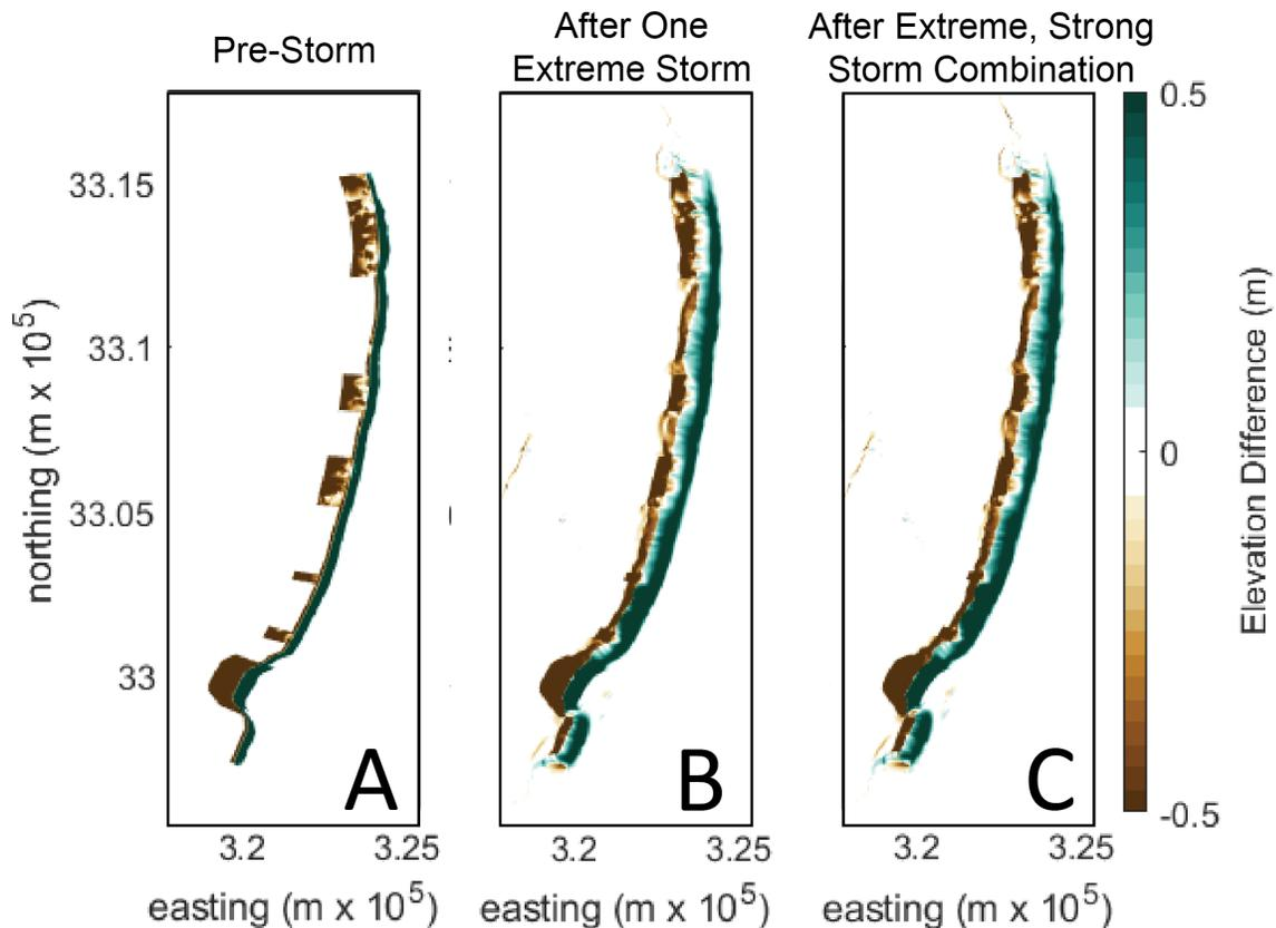
**Figure 50. Difference between the dune and marsh restoration templates before (A) and after an extreme storm (B) and a strong storm after an extreme storm (C). Positive (green) values indicate the dune template is higher in elevation, negative (brown) values indicate the marsh template is higher in elevation.**
