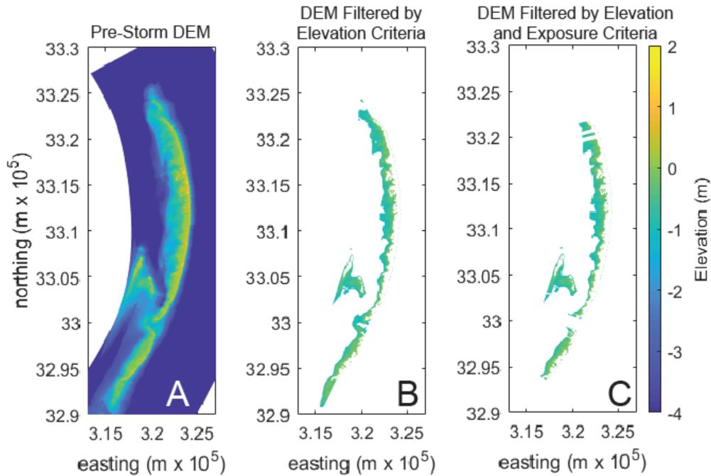
**Figure 33. Calculation methodology for potential seagrass area (Asg). The DEM (A) is first filtered to retain only those elevations that fall between -0.17 m and -1.31 m MLW (0 m to -1.15 m NAVD88). A second filter is then applied to remove those areas that are not protected by a subaerial island, defined as having elevation points higher than 0.04 m MLW (0.21 m NAVD88).**
