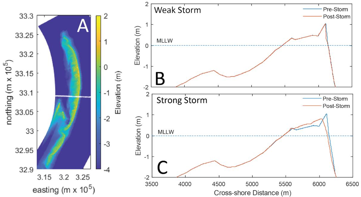
**Figure 38. (A) Pre-storm DEM and the pre- and post-storm cross-shore elevation for the transect shown in white. Results are shown for a weak (B) and strong (C) storm with SE waves.**
