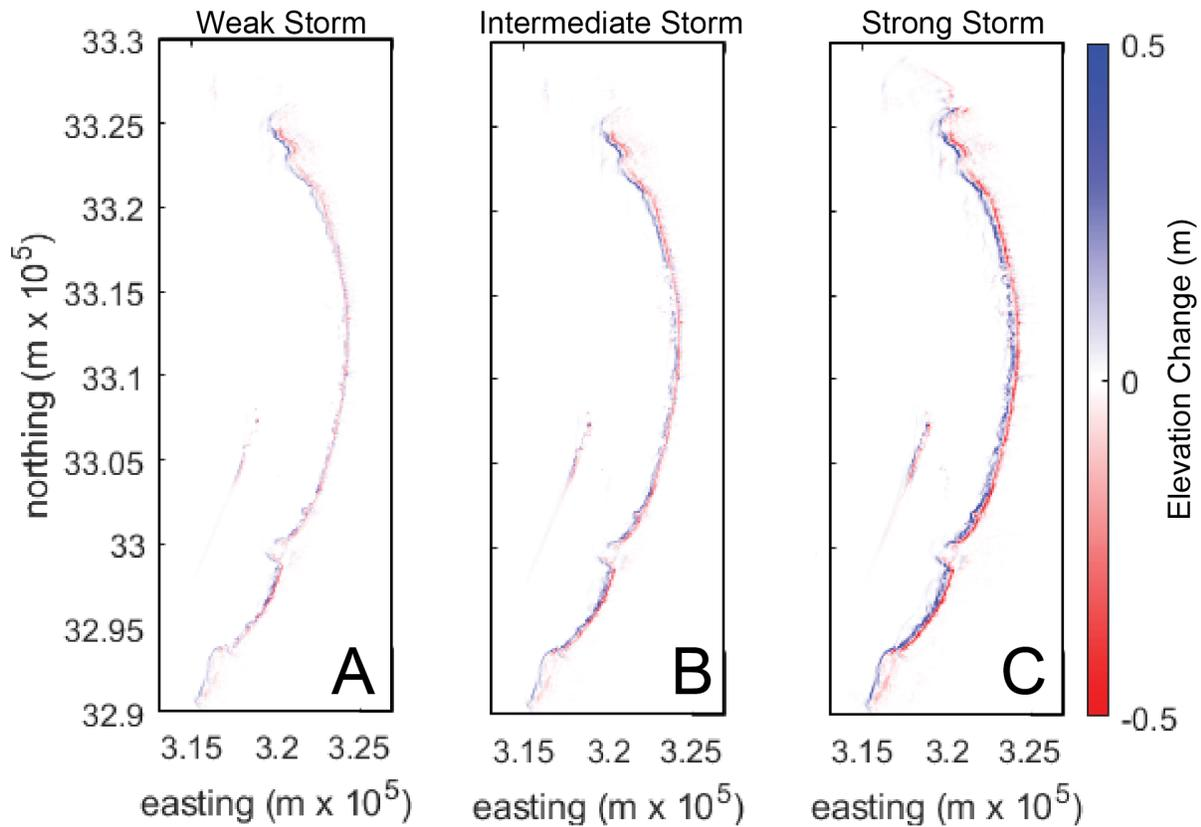
**Figure 36. Elevation change resulting from a weak (A), intermediate (B), and strong (C) storm. Storm characteristics are provided in Table 3.**
