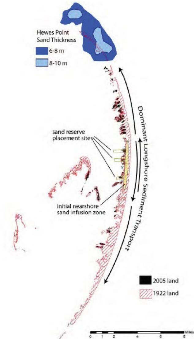
Figure 21. Conceptual design for Chandealeur Island restoration from Lavoie et al. (2009) involving backbarrier sand feeders placed in the central portion of the island arc constructed using sand from Hewes Point.
