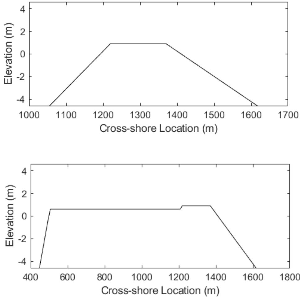
**Figure 26. The marsh end member restoration template. Top: Beach only template that is applied to most profiles. Bottom: The beach with backing marsh template that is applied where there is existing marsh.**
