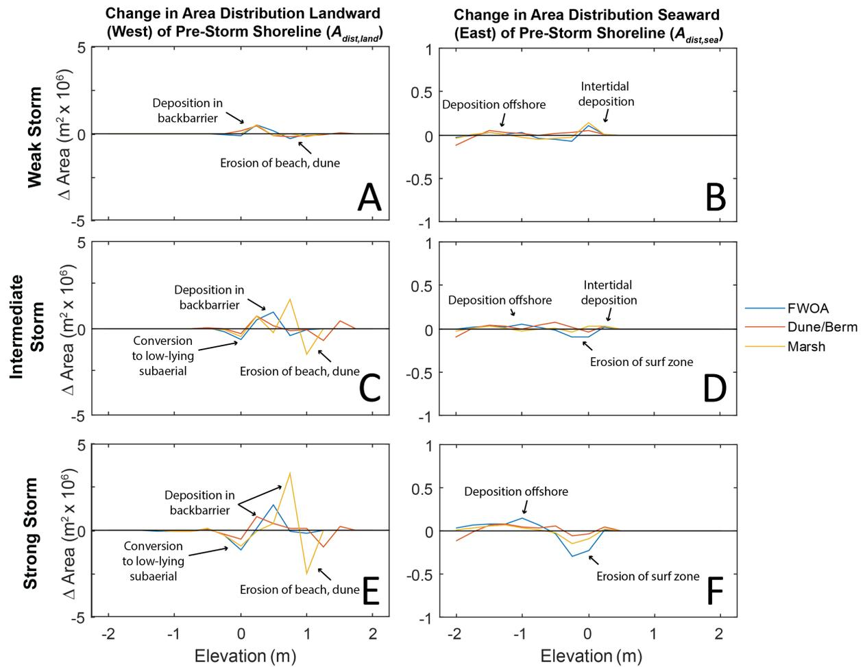
**Figure 45. Change in distribution of shallow and subaqueous elevation by area ( $A_{dist}$ ) for three alternatives including future without action (FWOA), placement of sediment on the dune and berm, and placement of sediment in the backbarrier marsh. Shown is the change in distribution of elevation landward (left column) and seaward (right column) of the pre-storm shoreline for a (A,B) weak, (C,D) intermediate, and (E,F) strong storm.**
